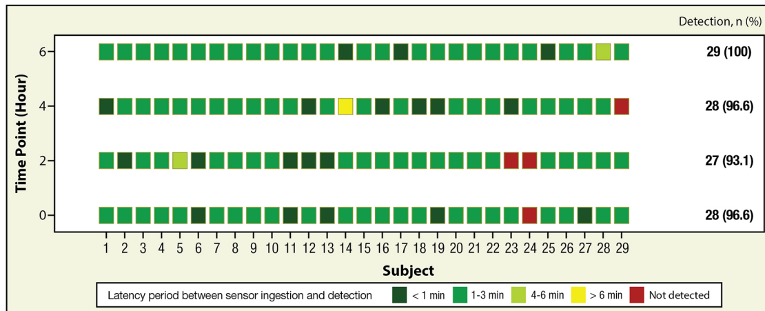
Figure 3. Detection of Ingestible Sensor by Wearable Sensor and Latency Period From Ingestion to Detection by Wearable Sensor in Individual Subjects at Each Time Point in Substudy B a
